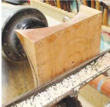
▲ Pic.20 Next, mount the bowl in the chuck jaws. Mark the diameter of the bowl and position the toolrest so it is straight across the front – this acts as a guard
